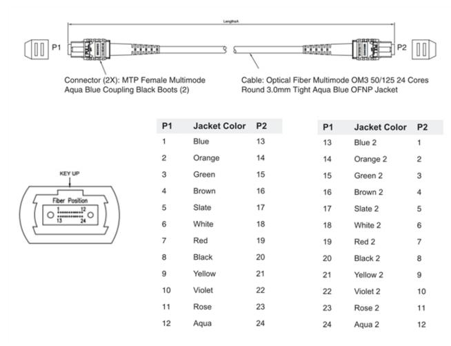
Figure 29 MPO/MTP 24 Position Fiber Cable
